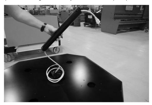
3. Thread the Lower Adjustable Mast section into the base plate and tighten the set screw using the provided Allen Key (Part E).
